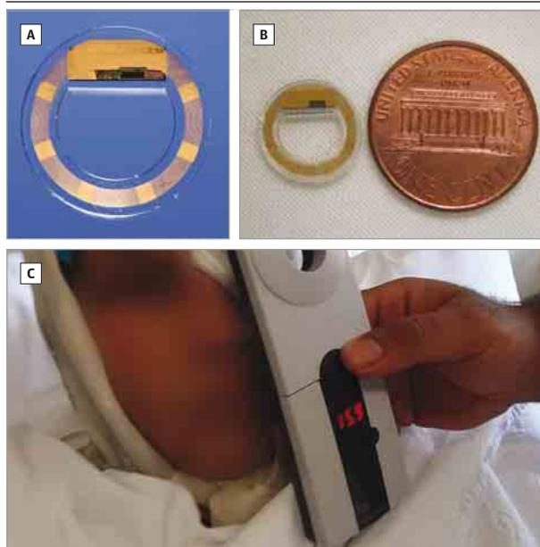
A, The device is encapsulated in silicone and has an 11.3-mm outer diameter and a 7-mm inner diameter. B, A view of the WIT showing its relative size alongside a US cent. C, The external reading device is held no farther than 5 cm from the transducer. It allows intraocular pressure (IOP) measurement by radiofrequency and displays an IOP reading representing the average of 10 to 20 IOP measurements.
