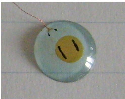
**Fig. 2** Sanchez's IOP sensing contact lens using a piezoresistive bilayer membrane. Image provided courtesy of author [56]
