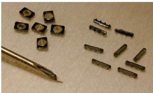
**Fig. 6** Different conformations of implantable unpowered parylene MEMS intraocular pressure sensors. Size is compared to a 19 gauge needle (left) [65]
